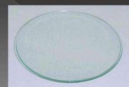
8.) Evaporating dish-is a laboratory device for evaporation of solids and supernatant fluids, and sometimes to their melting point. Evaporating dishes are used to evaporate excess water - or other solvents - to ensure that a concentrated solution or the dissolved substance is left behind.
