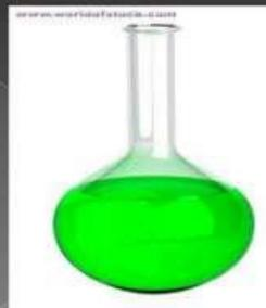
, also known as a conical 4.) Erlenme flask, is a widely used type of laboratory flask which features a flat bottom, a conical body, and a cylindrical neck. Erlenmeyer flasks are suitable for heating liquids. he small neck reduces evaporative losses compared to a beaker, while the flat bottom of the conical flask makes it unlikely to tip over and spill.
