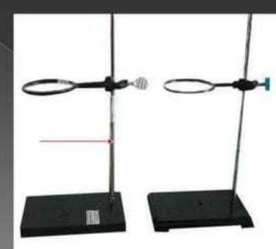
13.) Iron stand A metal rod attached to a heavy metal base. The heavy base keeps the stand stable, and the vertical metal rod allows for easy height adjustment of the iron ring/Clamp. (A tripod can sometimes be used in place of an iron stand)
